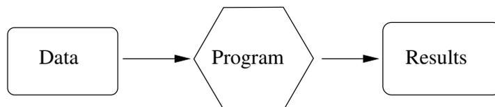
The “program” in the figure can be either a compiled program<sup>1</sup> (such as `ls`), or it may be *interpreted*. In the latter case, a machine-executable program such as `awk` reads your program, and then uses the instructions in your program to process the data.
